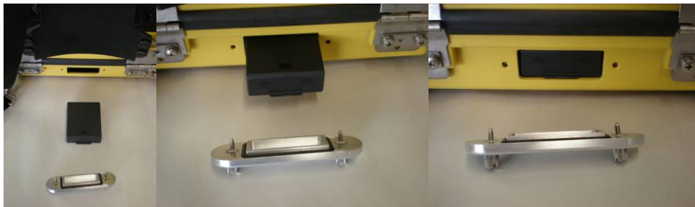
Figure 5: Installation of Battery Pack into CHTX transmitter
