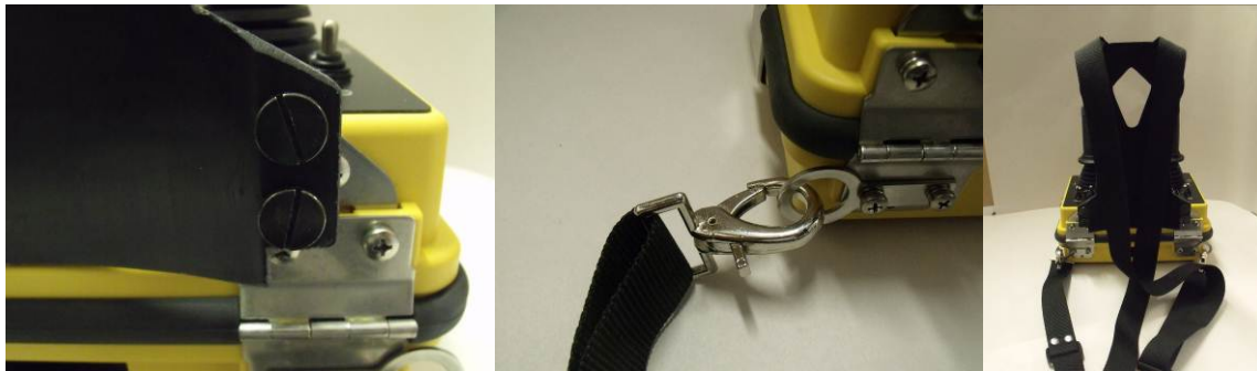
Figure 2: Chest Plate Installation
