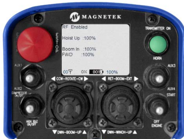
Figure 5: Machine Stop Switch and START push button
